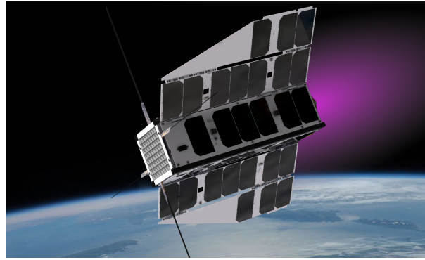
Figure 1: Artist's impression of an ABEP CubeSat in orbit. The graphics are an adaptation of the “Kelpie” 3U CubeSat from AAC Clyde Space [1]. Picture of the Earth by NASA/ISS Expedition 55. The atmospheric intake is visible as the grid aperture in the front of the spacecraft.
